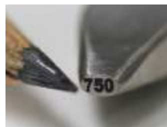
Micro Engraving on Hardened SS
