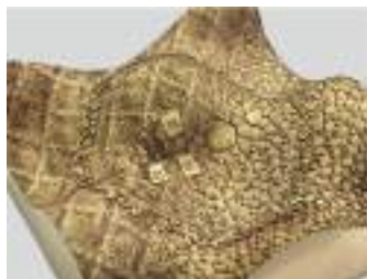
Engraving & Texturing on Freeform Surface
