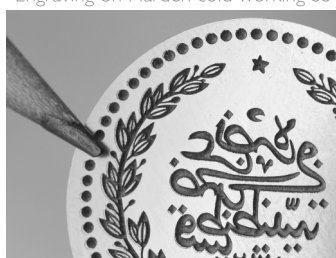
Engraving on Harden cold working SS
