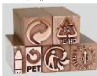
Deep Engraving on Copper Electrode
