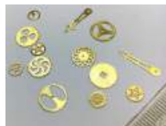
Micro Fine Cutting of Watch Part
