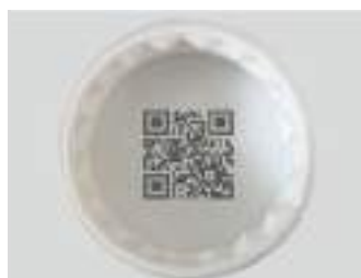
Laser Marking on Plastic Enclosure
